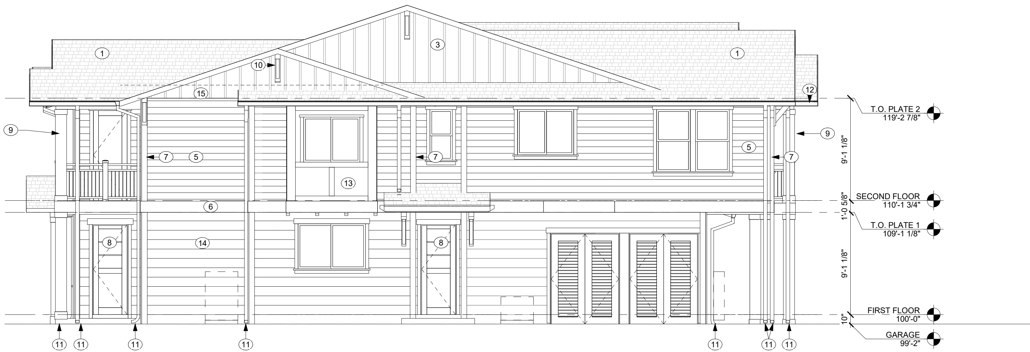
2 8-PLEX - CR - RIGHT ELEVATION MF8-4 SCALE: 3/16" = 1'-0"
