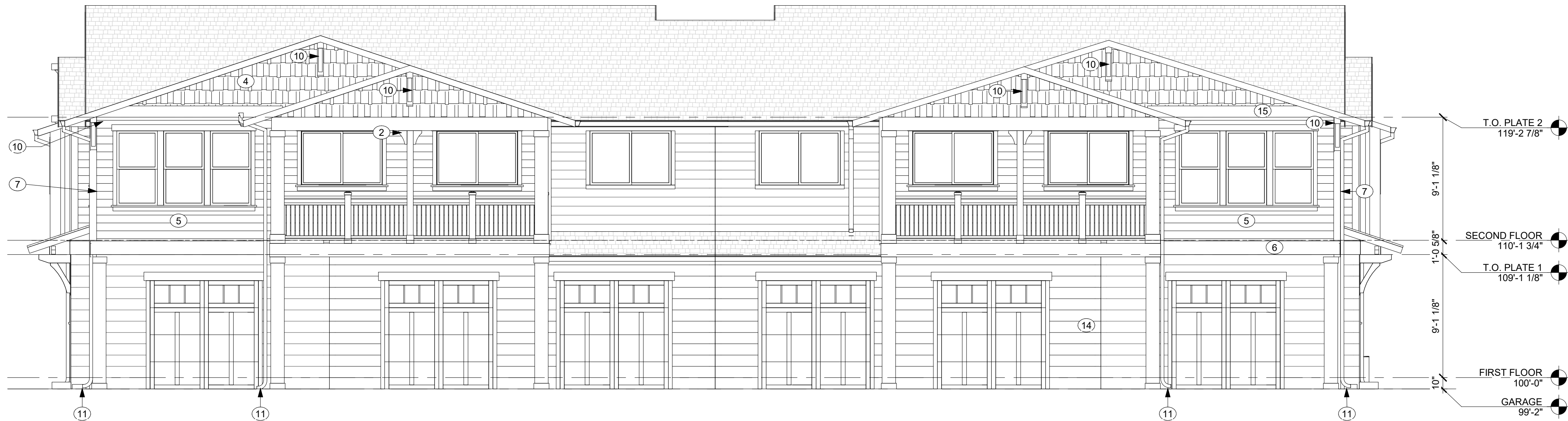
1 MF6-4 6-PLEX - CR - REAR ELEVATION SCALE: 3/16" = 1'-0"
