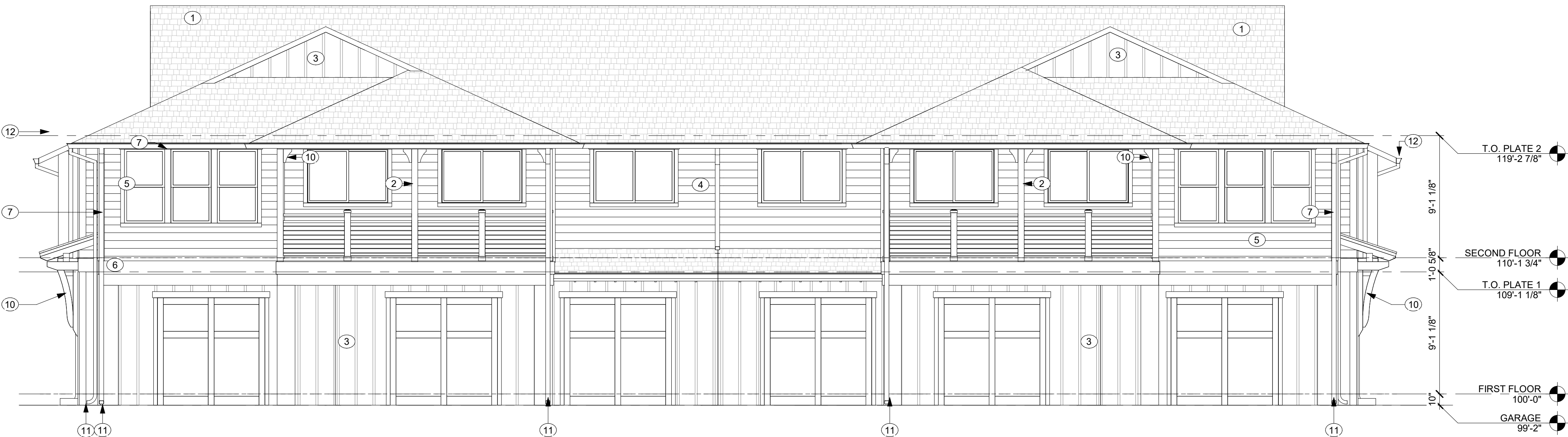
1 MF6-8 6-PLEX - PL - REAR ELEVATION SCALE: 3/16" = 1'-0"
