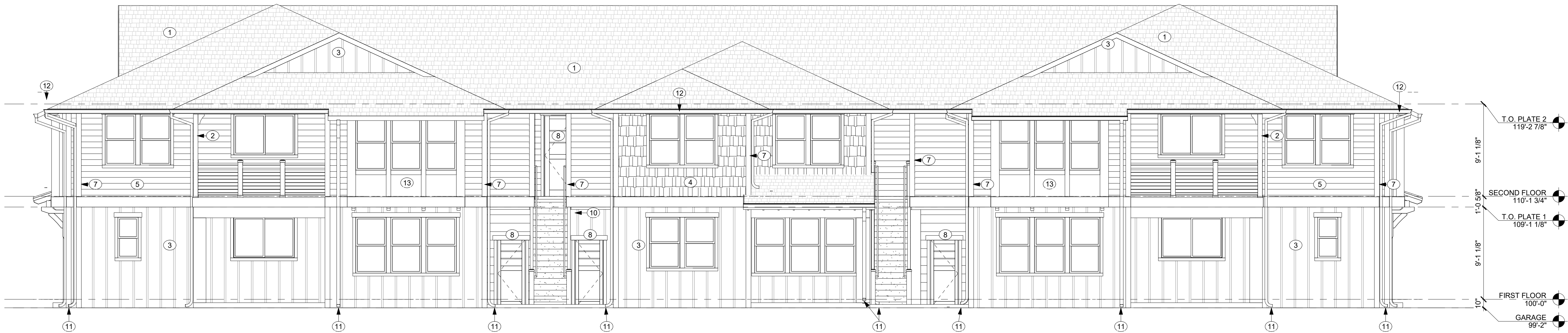
1 MF8-7 8-PLEX - PL - FRONT ELEVATION SCALE: 3/16" = 1'-0"
